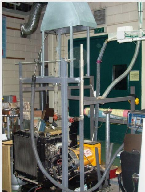
We control engine speed and engine load
